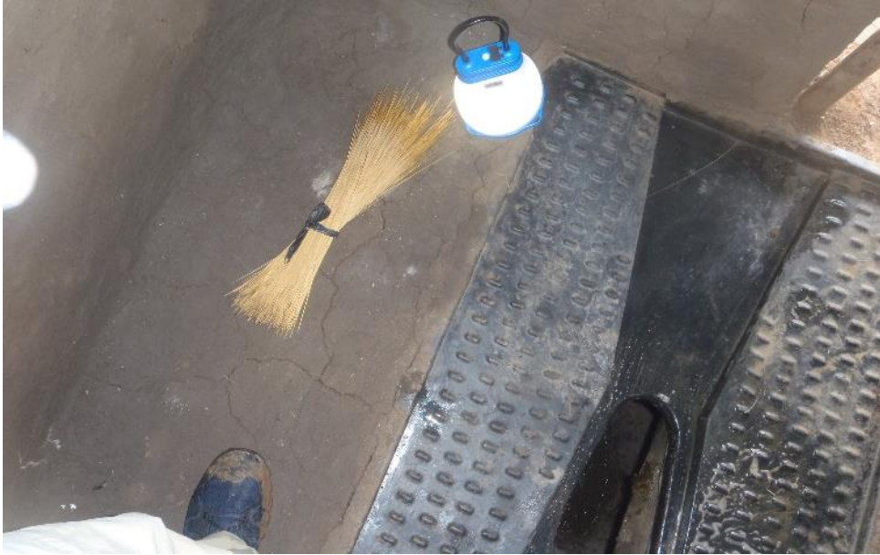
A UNHCR lantern in a household latrine. UNHCR distributed these SunBell Solar Lanterns – solar LED lights with a phone charger, 3m cable, solar disc and sound amplifier. They use a LiFe PO4 battery with 4–6 year lifespan. This battery charges in 4–10 hours, depending on the weather. The lamp has three settings: a full charge lasts 4.5 hours at 100 lumens, 15 hours at 20 lumens and 100 hours at 5 lumens. Photos: Brian Reed
